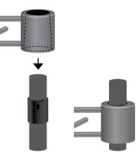
Slide the wire frames onto the clips. The attachments have a slight v-shape. The wider part has to point downwards.
